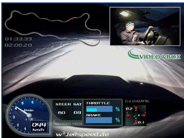
An example screenshot of a Video VBOX Lite scene, showing Speed, G-Force and track position overlaid onto a DVD quality recording of driver and vehicle
