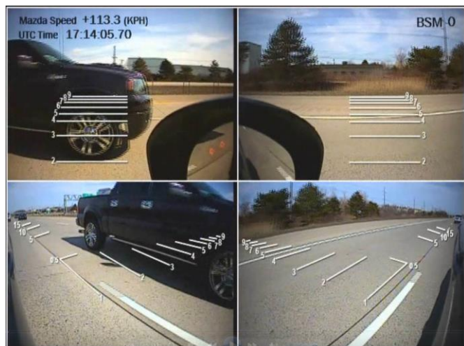
Video VBOX 4 camera system used to test Blind Spot Detection
