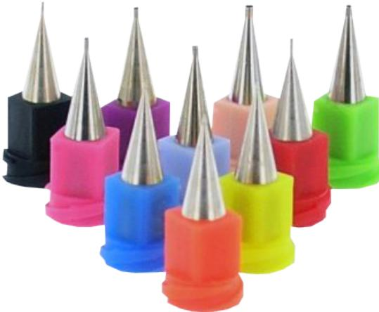
The conical form of these needles makes it possible to let the fluid easily flow with a progressive reduction and loss of charges. The result is that there is a bigger flow than when you use a stainless cannula needle for an identical pressure. Hereby you can work with less pressure in order to manage the material.
