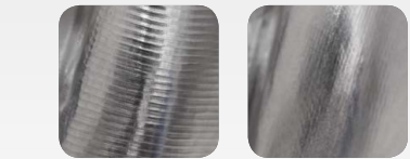
Surface achieved without (left) and with smoothing filter (right)
