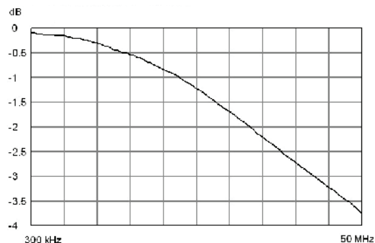
Insertion Loss Plot For 40-530-021 (typical worst case)
