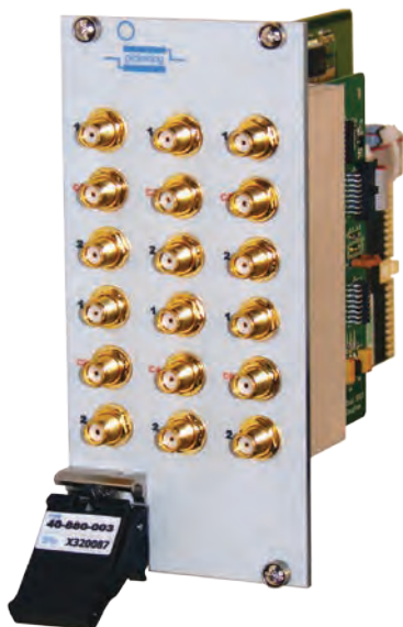
40-880-003 Hex SPDT Terminated 6GHz Switch
