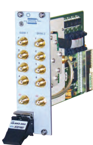
40-882-002 Dual SP4T Terminated 6GHz MUX
